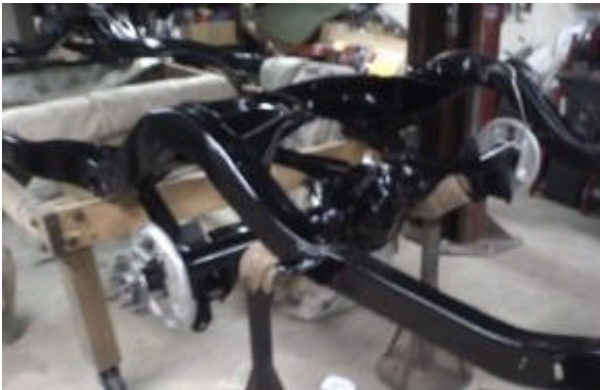
Larry's frame after installing the rear end 1-21-09
